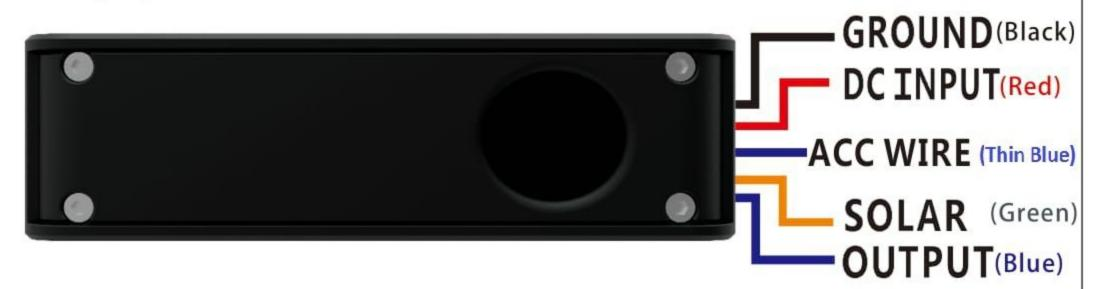
Using the twin core wiring laid between the main starting battery and the DC-DC charger, connect the red (+) to the (+) DC input terminal and the black (-) to the (-) shared negative on the rear of the charger. Finally, make the power connections to the main starting battery of the vehicle. It is recommended to install a 25 Amp circuit breaker (not included) as shown on main diagram. The circuit breaker should be located close to the starting battery.
