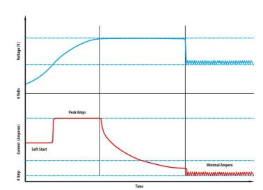
Charging algorithm will change according to battery type.
